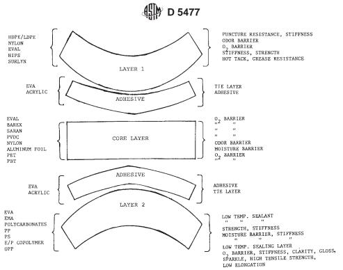
FIG. 1 Position and Function of Materials in Typical Multilayer Films
